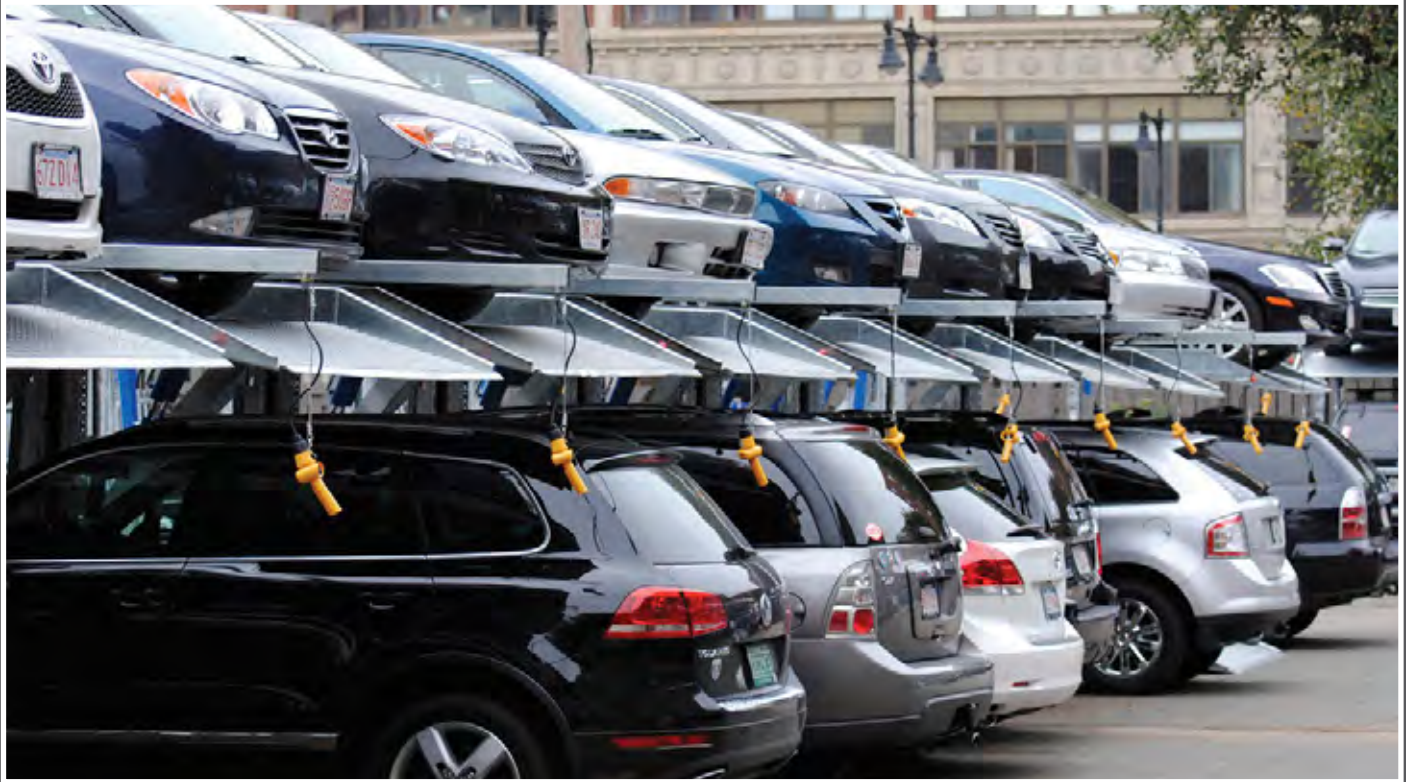
2-POST, 2-LEVEL VEHICLE LIFT FOR STACKING CARS
