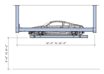
SP100 Suspended Platform can be ceiling-hung or integrated into building structure.
