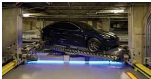
STORAGE: Vehicle is automatically parked by Rack & Rail System
