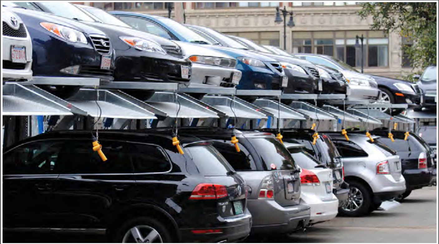
2-POST, 2-LEVEL VEHICLE LIFT FOR STACKING CARS
