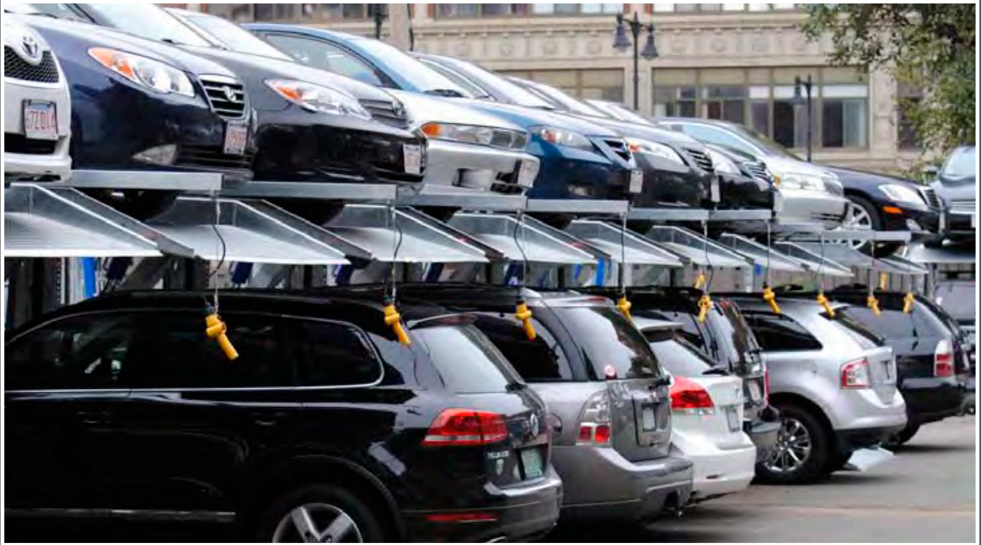
2-POST, 2-LEVEL VEHICLE LIFT FOR STACKING CARS
