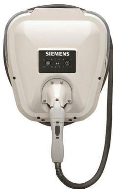
The **Siemens VersiCharge Electric Vehicle AC Charging Station** is a Level 2 (240 VAC) hardwired charging station that provides automatic charging when connected to an electric vehicle. The VersiCharge is typically post-mounted for SAPS and wall-mounted for APS. The EVSE (Electric Vehicle Supply Equipment) power output can be adjusted to match available electrical infrastructure at installation site.
